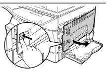
Check the misfeed location. Remove the misfed paper following the instructions for each location in the illustration below. If the error indicator blinks, proceed to "A: Misfeed in the paper feed area" (p.80).
